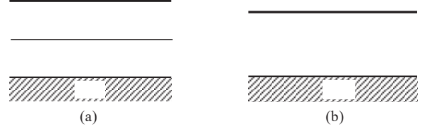
Fig. 1. Illustration of the concept of replacing a two-layer soil profile on bedrock with an equivalent single-layer soil profile.
